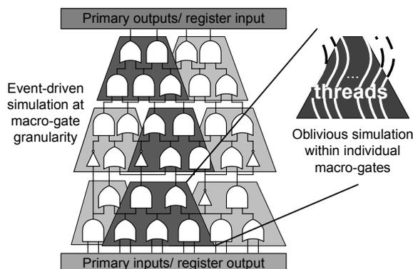
Fig. 2. **Hybrid event-driven simulator.** The GCS architecture is event-driven at the granularity of macro-gates, while the macro-gates themselves are simulated in oblivious fashion. As an example, during a simulation cycle, only the darker macro-gates could be activated, each of them simulated one after the other by a single thread block in an oblivious fashion.
