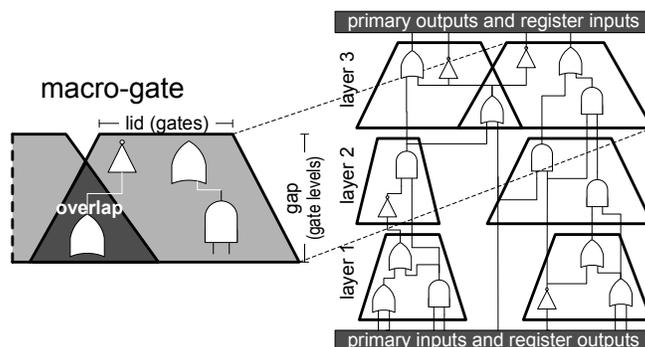
Fig. 4. **Macro-gate segmentation.** The levelized netlist is partitioned into layers, each encompassing a fixed number of gate levels (gap). Macro-gates are then carved out by extracting the transitive fanin from a set of nets (lid) at the output of a layer, back to the layer’s input. If an overlap occurs, the gates involved are replicated to all associated macro-gates.
