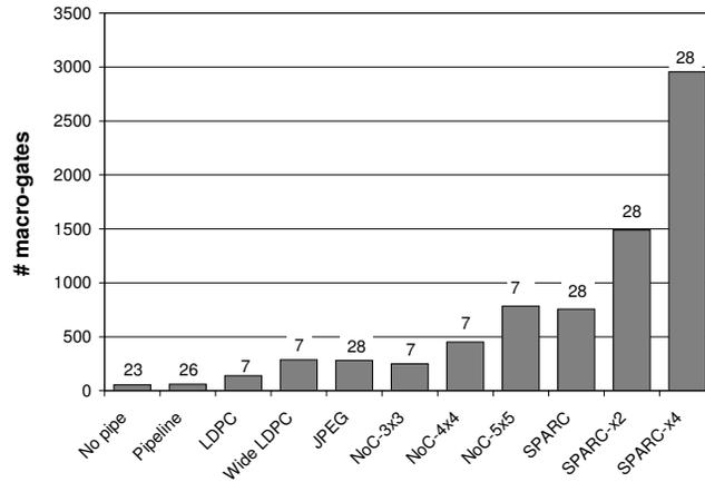
Fig. 14. **Number of macro-gates and layers.** The figure plots the total number of macro-gates for each design using the baseline segmentation algorithm. The value above each bar indicates the number of layers in the segmentation. Larger designs result in more macro-gates.
