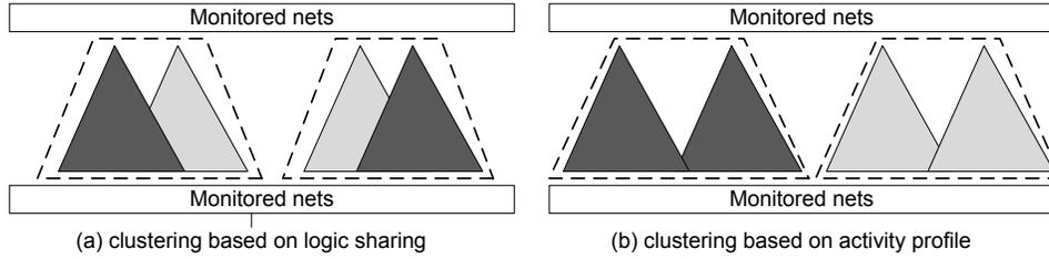
Fig. 9. **Profile-based clustering** compared to baseline algorithm. The baseline clustering algorithm (a) groups cones of logic by degree of logic sharing, while profiling (b) is based on the activation frequency of logic cones. In the picture a cone’s shading is proportional to its activation frequency. Clustering based on activity profile results in the consolidation of frequently activated logic cones.
