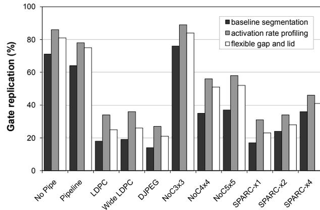
Fig. 15. **Gate replication during macro-gate segmentation.** The graph plots the increase in the number of gates in the design due to gate replication over all three segmentation algorithms discussed. The least replication is provided by the baseline algorithm.
