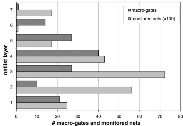
Fig. 16. **Geometry after baseline segmentation** for the LDPC design. For each layer we report the number of macro-gates as well as monitored nets in hundreds generated when segmenting the design according to baseline algorithm.
