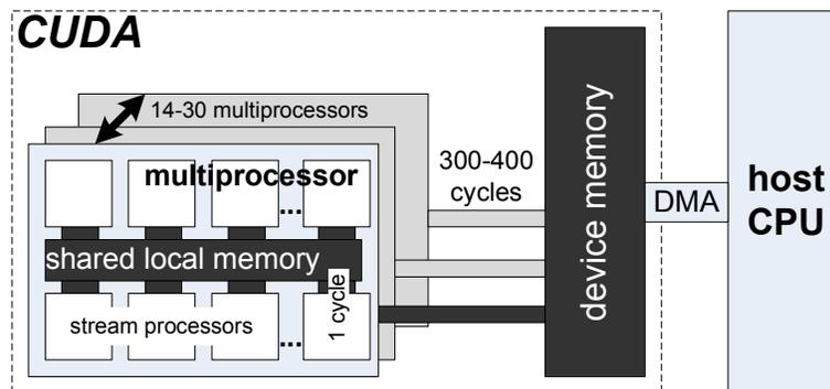
Fig. 1. **NVIDIA CUDA architecture.** The GPU contains an array of multi-processors, each containing individual stream processors. Within a multiprocessor, the stream processors have access to a small, fast shared local memory. Multiprocessors can also access higher latency device memory. Finally, the GPU device communicates with the host CPU via DMA.
