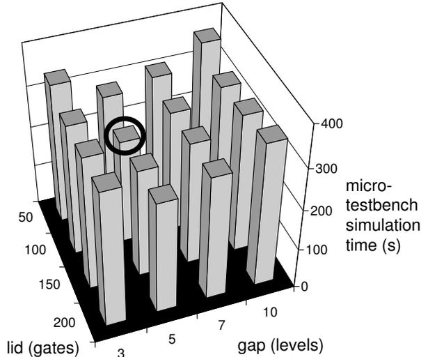
Fig. 8. **Ideal gap and lid estimation** for the LDPC testbench design. The figure shows the runtime for a micro-testbench simulation using a range of gap and lid values. The ideal gap and lid values, achieving minimum simulation time within the range considered, is highlighted by the dark circle.
