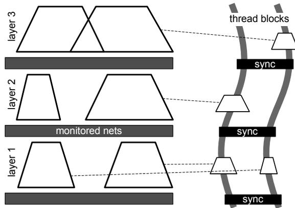
Fig. 10. **Event-driven simulation** proceeds layer by layer at the macro-gate granularity. Within each layer, activated macro-gates are simulated and monitored nets are analyzed to determine which subset of the next layer's macro-gates should be activated. Activated macro-gates are transferred by the CUDA scheduler to an available multiprocessor for simulation.
