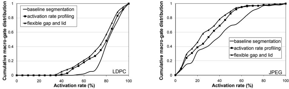
Fig. 20. **Cumulative distribution of macro-gates** with respect to activation rates for LDPC and JPEG designs. The plot shows the trends for all three segmentation heuristics presented: baseline segmentation, activation rate profiling and flexible gap and lid. The flexible gap and lid heuristic performs the best with the greatest improvement on macro-gates with low activation rates.
