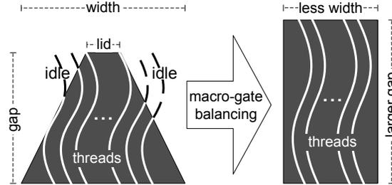
Fig. 6. **Macro-gate balancing.** The balancing algorithm restructures each macro-gate to minimize the number of execution threads required. The result is a more efficient utilization of thread block resources.
