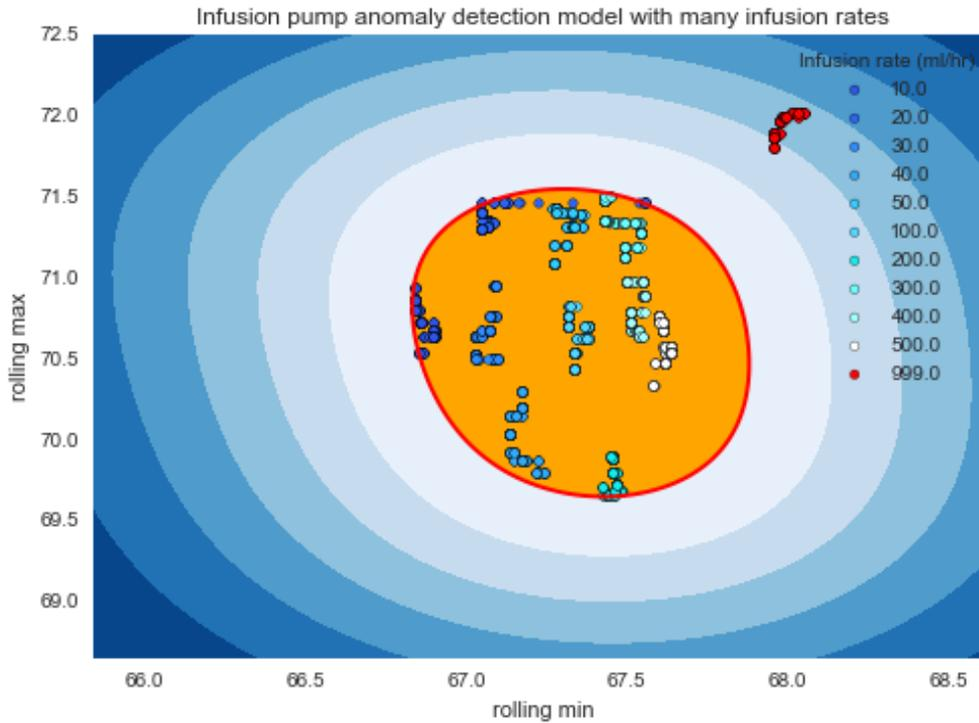
Figure 4: CareFusion Alaris 8100, multiple normal infusion rates (10 ml/hr to 500 ml/hr, white dots) vs. abnormal 999 ml/hr (red dots)
