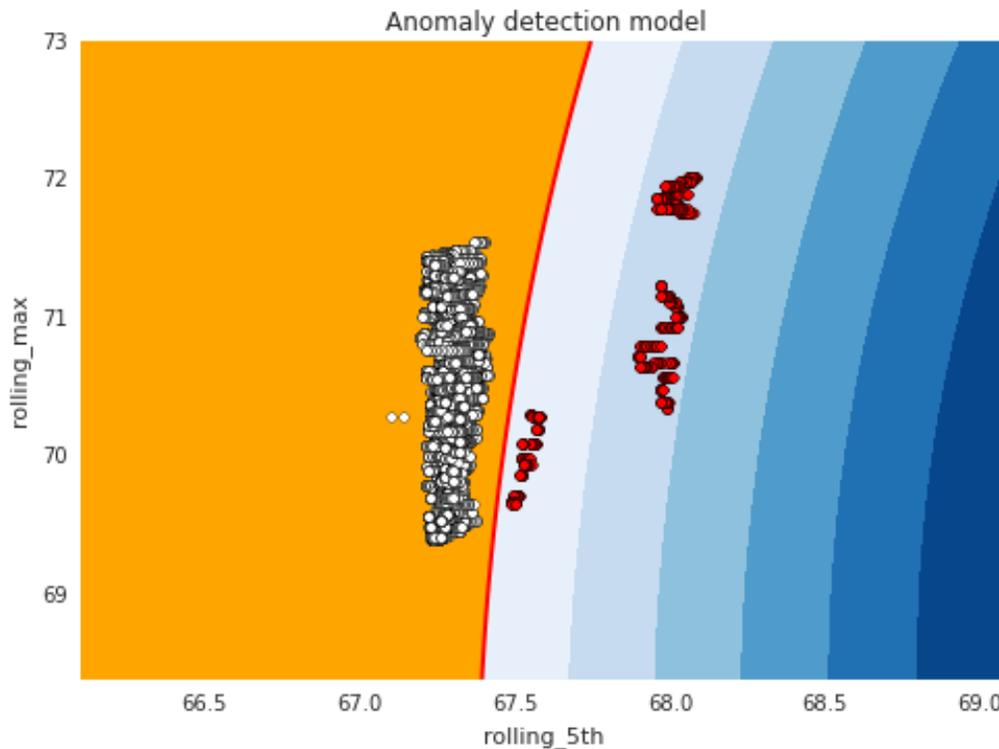
Figure 7: CareFusion Alaris 8100. Training on both normal and abnormal datasets. Normal infusion rate of 10 ml/hr (white dots) compared to the attacker scenario of 500 ml/hr and 999 ml/hr (red dots).
