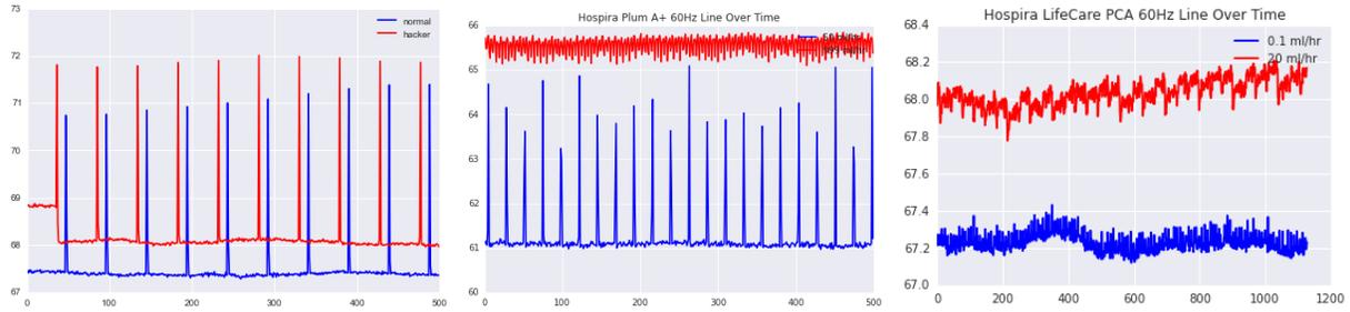
Figure 2: Amplitude of the 60 Hz band, which is directly proportional to power consumption caused by electromechanical actuation (pumping). Left: Alaris 8100 pump with 8015 PC. Middle: Hospira Plum A+. Right: Hospira Lifecare PCA. In all plots, blue represents a “normal” infusion rate (50 ml/hr for Alaris 8100 and Hospira Plum, 0.1 ml/hr for Hospira PCA). Red represents an “abnormal” infusion rate (999 ml/hr for Alaris 8100 and Hospira Plum, 20 ml/hr for Hospira PCA).
