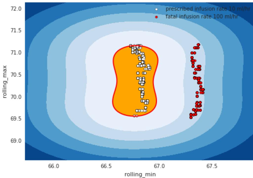
Figure 6: CareFusion Alaris 8100. Normal infusion rate of 10 ml/hr (white dots) compared to abnormal infusion rate of 100 ml/hr (red dots).
